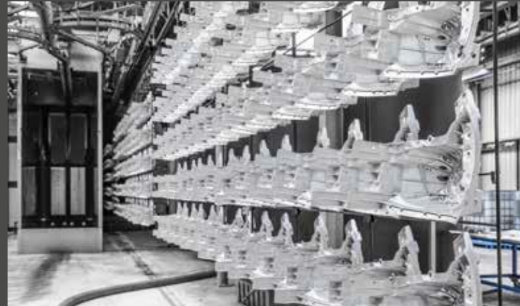
PRETREATMENT: Degreasing and etch passivation using Alodine 2040R2.
