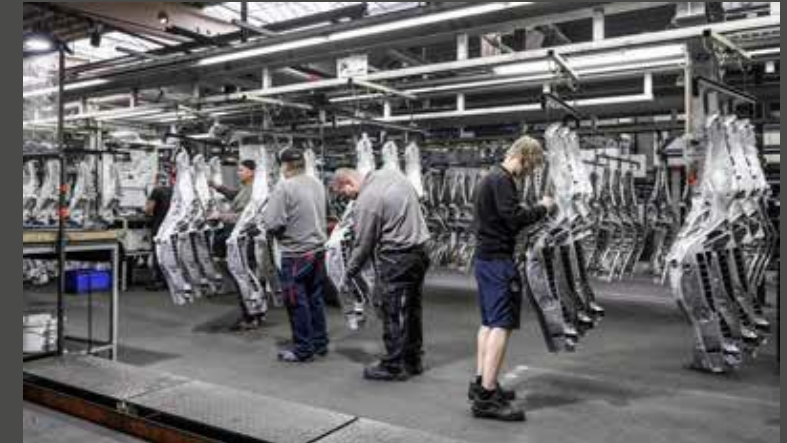
Hanging of components and masking of areas to be left unpainted
